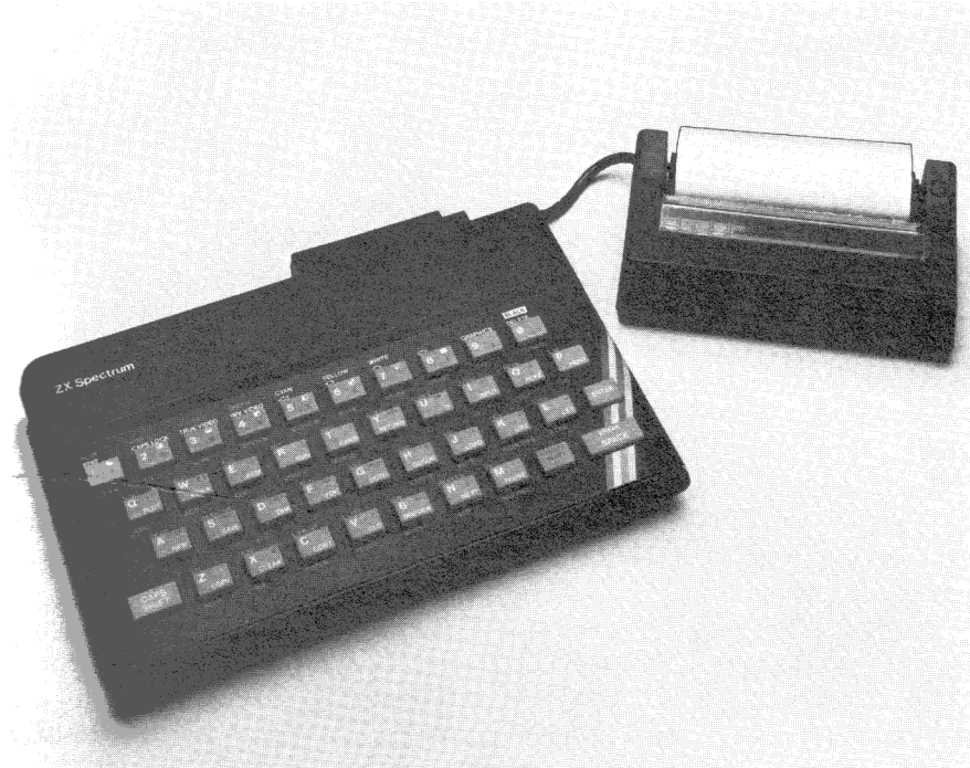
Figure 1.6 A printer attached to the ZX Spectrum.
